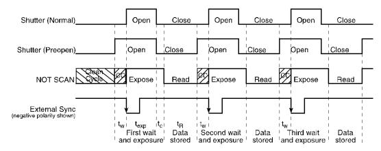
Figure 20. Continuous Cleans Timing Diagram (- edge trigger)
